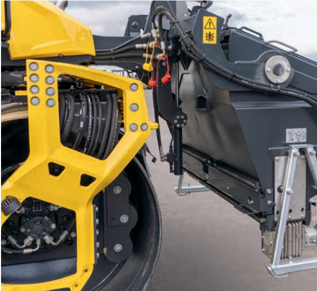
BS 150 and BS 180 precision spreaders are suitable for all conventional chippings, including double-crushed chips 2/5 and 1/3 particle size as well as crushed sand particle size 0/2.
